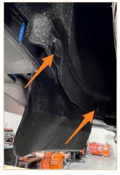
3. On the inside of the front bumper, unplug the marker lights (one on each side) and the front bumper harness connector.
