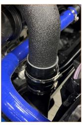
35. Reinstall the diverter valve hose and secure it with the stock clamps.
