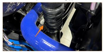
22. Remove the lower section of the hot side charge pipe out through the bottom.
