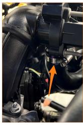
25. Remove the 2 nuts from the hot side charge pipe flange (10mm socket) then remove the upper section of the hot side charge pipe. It will have to be rotated 180 degrees to get it around the harness.
