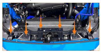
7. Behind the grill shutters and in front of the radiator, remove the screw for the grill shutter link (5.5mm socket), then bend the 2 tabs out on the bottom end and remove the link.
