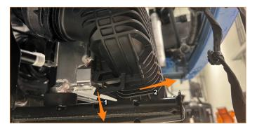
18. Lift on the bottom of the radiator until the rubber mounts, clear the holes, and then swing the bottom of the rad forward. This will give clearance to get the charge pipes in and out.
