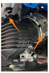
17. Release the intercooler from the radiator by pulling down on the lock tabs and then pulling forward on the bottom of the intercooler. Remove the intercooler by lifting the whole assembly up over the hooks on the radiator then removing it out the front. Note: you may have to lift up on the AC condenser.
