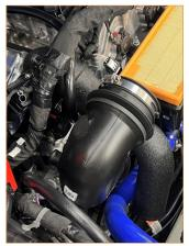
29. Slide an 89mm worm gear clamp onto the charge pipe, then install coupler 1. Place an 89mm worm gear clamp over the lower section of the Mishimoto charge pipe, then install it onto the coupler through the bottom side of the vehicle.
