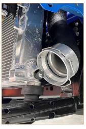
31. Move the radiator mounts back into their mounting positions.
