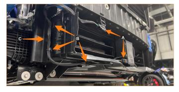
10. Remove the 4 bolts fastening the grill shutter assembly and the 4 bolts for the lower brace (8mm socket).
