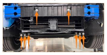
11. Unplug the electrical connector "A", remove the 3 harness tree clips "B", and remove the 2 bolts "C" (8mm socket). Remove the grill shutter assembly and the lower brace from the vehicle.
