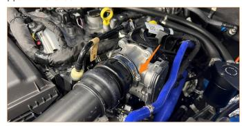
20. Unplug the electrical connector for the MAF sensor, loosen the clamp on the intake pipe (7mm socket), then release the 3 clips on the airbox top and remove it.
