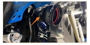
23. Unplug the electrical connector, and then remove the 3 harness clips.
