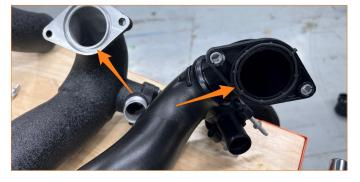
28. Install the upper section of the Mishimoto charge pipe in the vehicle by feeding the bead rolled end under the harness and rotating it into position onto the mounting studs.
