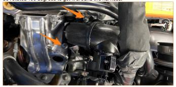
26. Remove the 3 screw studs from the stock hot side charge pipe. Swap the diverter valve to the Mishimoto charge pipe and fasten it with the provided M6 bolts.
