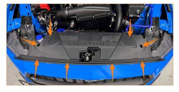
5. Behind the upper part of the front fender, remove the 2 bolts from the left-side front bumper bracket (10mm socket). Repeat for the right side.
