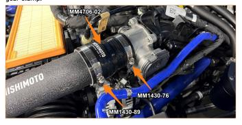
34. Fasten the upper section of the hot side charge pipe using the 2 stock nuts. Tighten the 2 89mm worm gear clamps on coupler 1.
